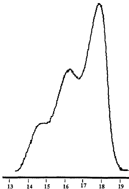
Figure 1. Molecular weight distribution of poly(2-vinylpyridine) prepared by initiation with t -BuLi in toluene at -78^{\circ}\text{C} . DP_n = 38 ; M_w/M_n = 2.7 ; [\text{t-BuLi}] = 2.5 \times 10^{-3}\text{ M} .
